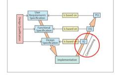
Before equipment can be used routinely in production, it must first be commissioned and, if necessary, undergo Installation Qualification (IQ). This module describes commissioning and IQ requirements and procedures in the medicines and healthcare products industries. It follows the activities of a typical validation team as they carry out a project for a pharmaceutical company.
